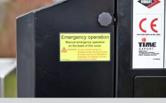
The shaped profile ultra high strength steel booms provide improved rigidity, stiffness and performance Ground level emergency lowering from the chassis (pedestal mounted valve bank)
