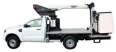
Emergency operation from ground (valve-bank mounted on pedestal)
