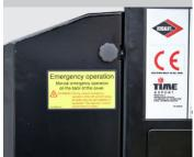
Ground level emergency lowering from the chassis (pedestal mounted valve bank)
