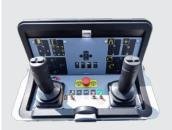
LMC (Load Moment Controls): Variable outreach and up to 2 actions at a time (1 per joystick)
