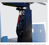
Ground level emergency lowering from the chassis (pedestal mounted valve bank)
